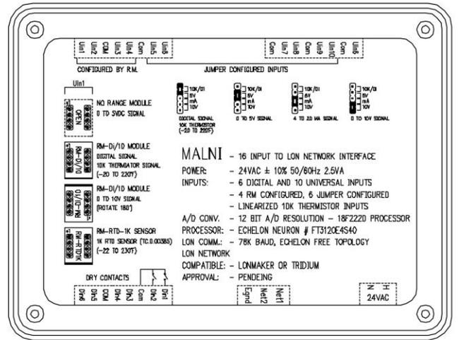
TYPICAL WIRING DIAGRAM
